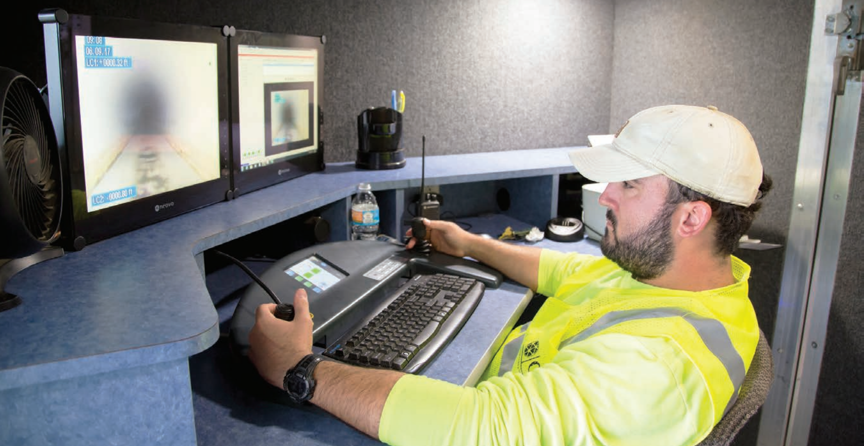
ABOVE Justin Ayers performs a CCTV inspection of a sewer line in Baton Rouge.
